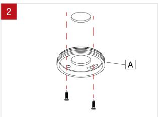
Locate the place the fixutre will be installed and make a 7/8" dia hole for the power cable to pass. Install the Threaded Adpater plate (A) with the screws where the hole was made.
