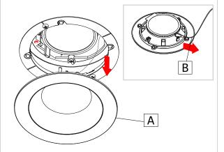
For trim installation, detach trim (A) from ceiling and unhook from safety wire (B). Safely store it on the side.
