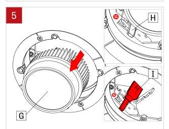
Push tab (H) on the side of the light element (G) to release it from the adjusting mechanism. Slide light element (G) from the track system (I).
