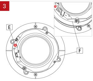
Slightly unscrew red screw (E) to allow vertical tilting of the adjusting mechanism (F).
