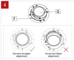
Align light element (G) straight by rotating and tilting the adjusting mechanism (F), in order to proceed with its removal in the next step.
