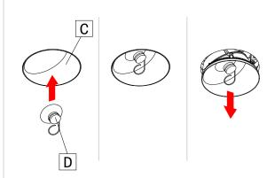
For trimless wall wash installation, detach baffle (C) by using provided suction tool (D). Stick tool on baffle lens and pull.
