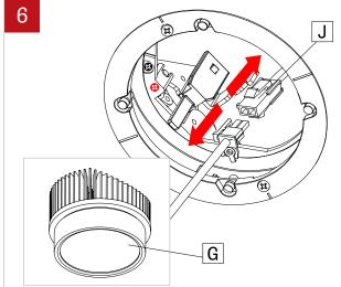
Disconnect the quick connectors (J) between the light element (G) and the driver.
