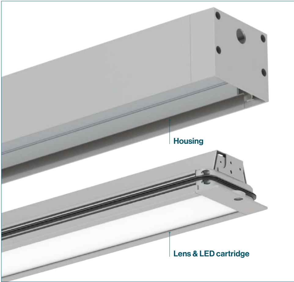
Sealed for continuous run Two adjacent individual sections are sealed by a silicone gasket attached to one of the two sections.
